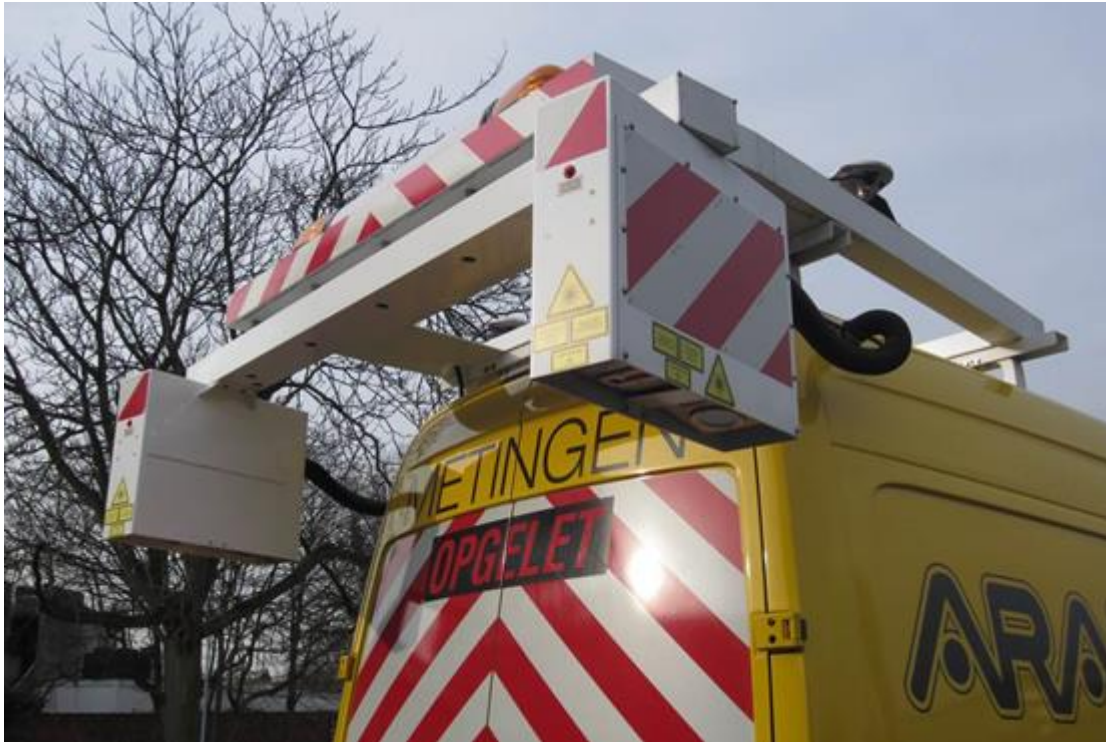
Figuur C.2 Laser Crack Measurement System (LCMS) op de ARAN.
